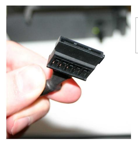
Identify the power supply connector for a SATA hard drive.
