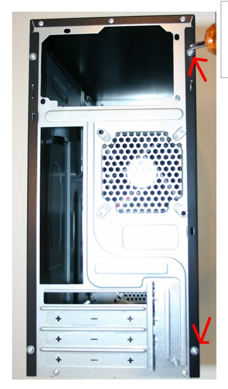
Turn the computer to face the back. Unscrew the two screws on the right where the red arrows point.
