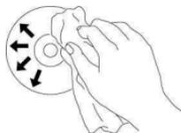
**CAUTION:** Do not use benzene, paint thinner, record cleaner, solvent or static repellent. This can damage the disc.
