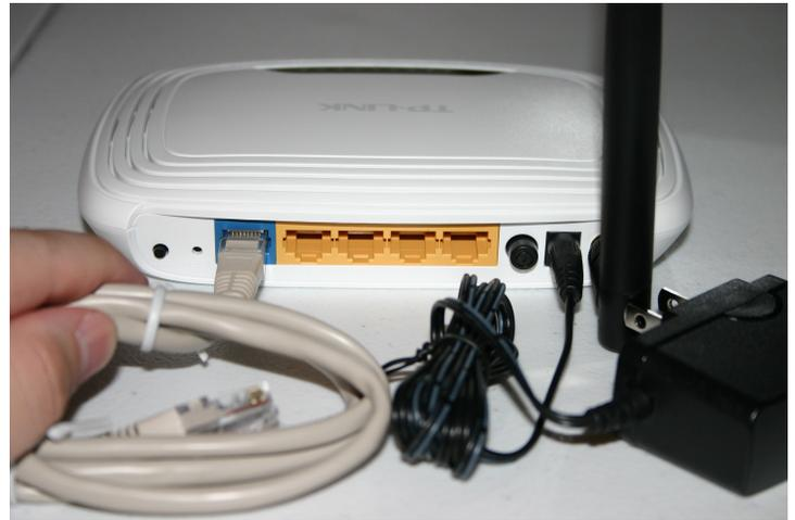
Step 3: Connect the ethernet cable to the blue WAN port
