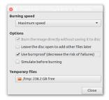
4. Click the Burn button to start burning. Make sure not to move the computer or DVD burner while the system is writing your image to disc. Doing so can result in failure.
