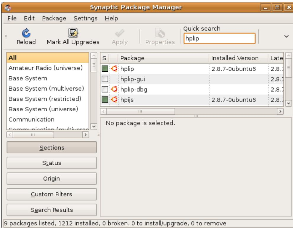
5. To mark the driver for installation click on the hplip-gui box
