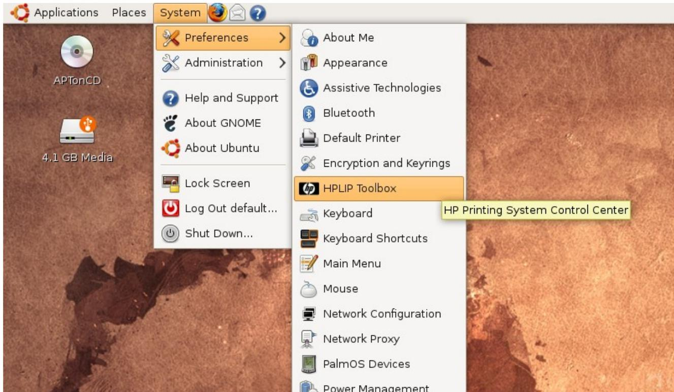
11. The first time you run HPLIP Toolbox you will be warned that no HP devices have been found, select Setup device... to detect and configure a newly connected device
